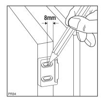
Remove the little plates and make the holes with a diam. of 2 mm. Replace the little platee over the runners and screw in the screws provided (3.5x16 mm).
